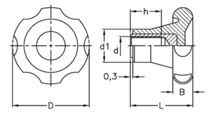
$\begin{array}{lll} B & = 13 \\ D & = 51 \\ d1 & = 23 \\ d \ 6H = M8 \\ h & = 13 \\ L & = 34 \end{array}$
